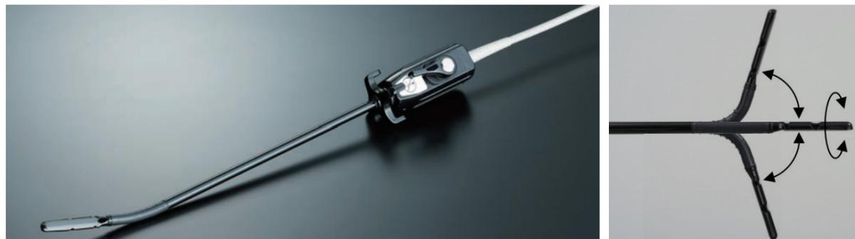
The transducer can be positioned with outstanding flexibility by bending and rotating the acoustic head.
