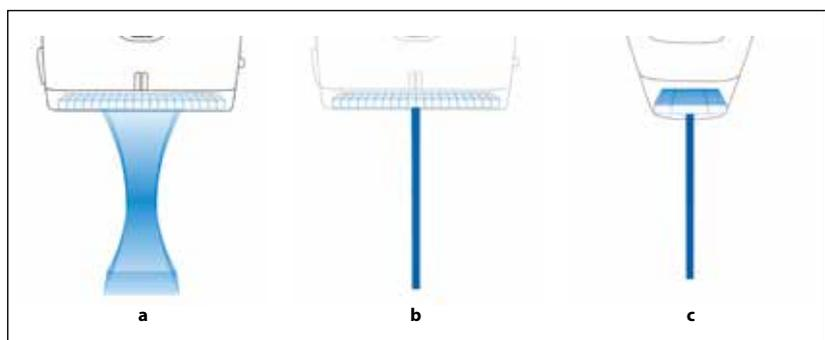
**Figure 2.** Conventional beam forming technology (a). iBeam forming technology produces a sharp, uniform and thin ultrasonic beam that offers clinical images with higher resolution, more homogeneity, and reduced artifacts (b). iDMS:iBeam-slicing in lens direction to enable continuous focus across all depths (c).
