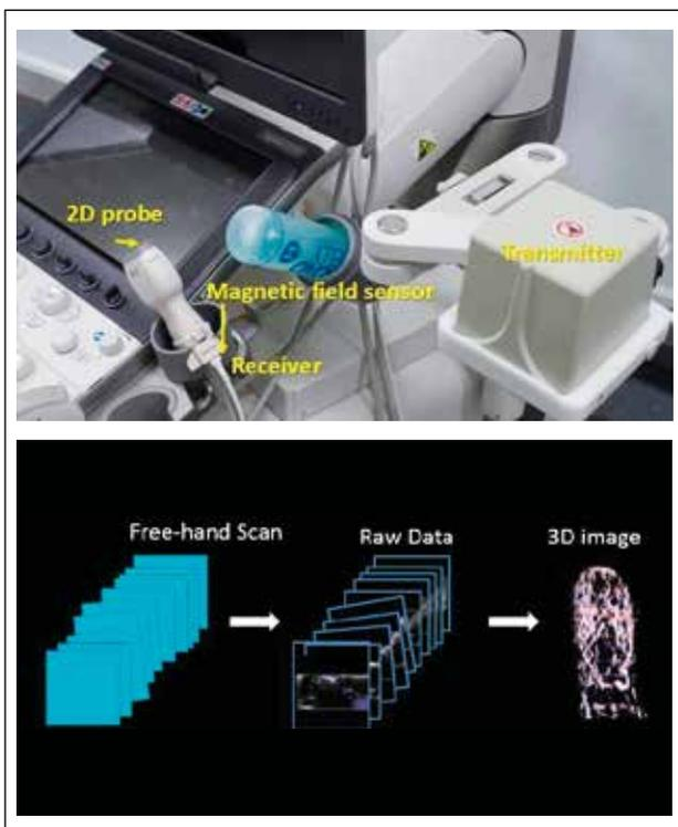
Figure 9. Basic principle of Smart Sensor 3D
