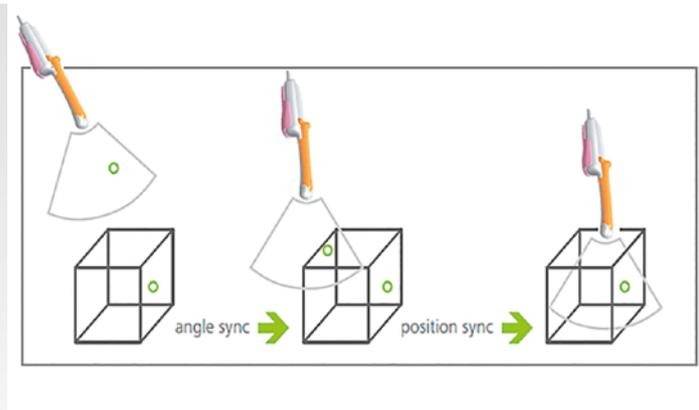
Fig. 1: Process of synchronising MRI and ultrasound images.
