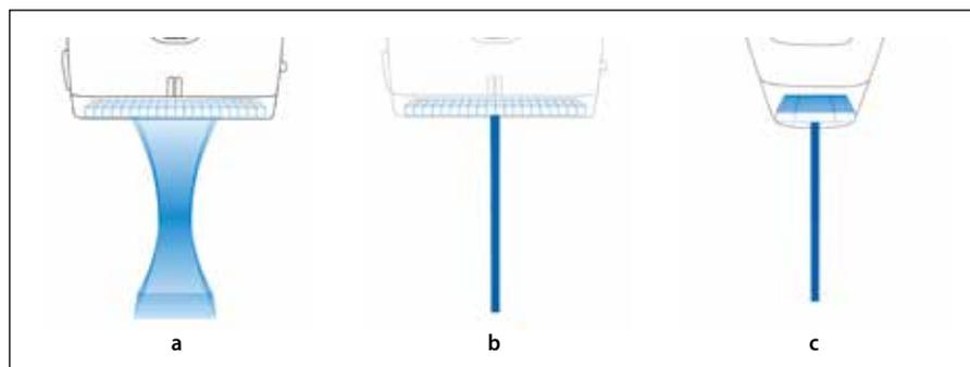
Figure 2. Conventional beam forming technology (a). iBeam forming technology produces a sharp, uniform and thin ultrasonic beam that offers clinical images with higher resolution, more homogeneity, and reduced artifacts (b). iDMS:iBeam-slicing in lens direction to enable continuous focus across all depths (c).
