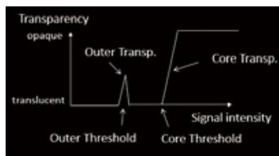
Figure 10. Principle of Shadow Glass
