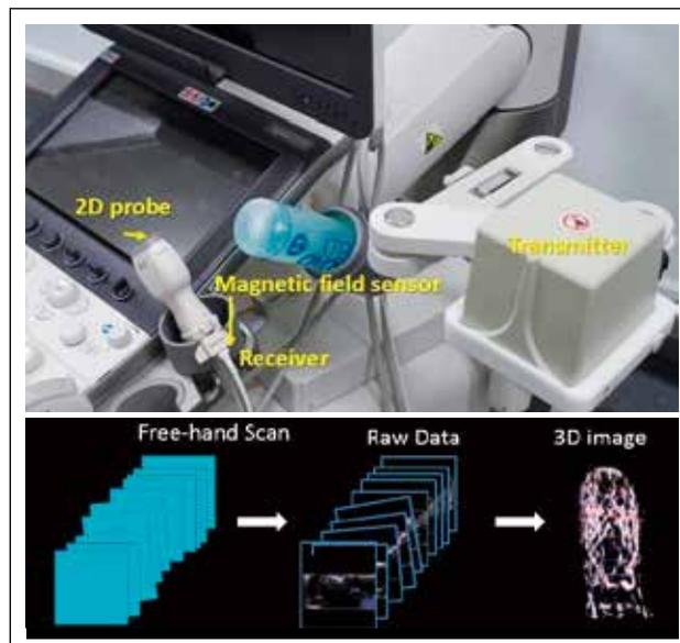
Figure 9. Basic principle of Smart Sensor 3D
