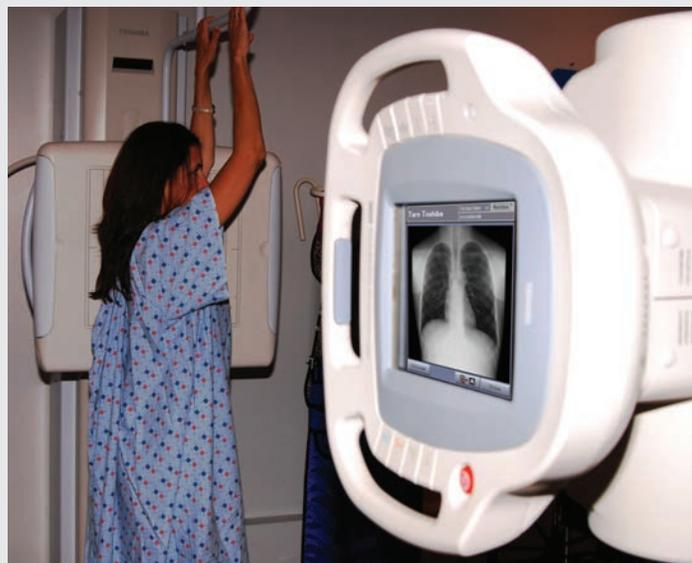
RexView, a color LCD screen on the overhead tube crane, displays real-time images so technologists can review on the spot, for faster decisions, without leaving a patient's side.
